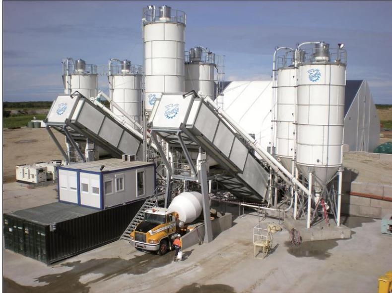
Figure 2 Double MMX plants installed on site for temporary production
