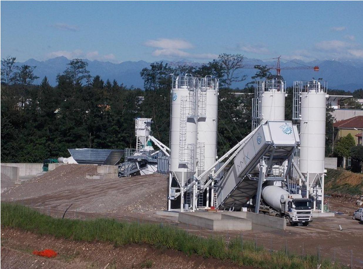
Figure 3 Highways in Italy – SIMEM Rental installation with 4 supermobile plants
