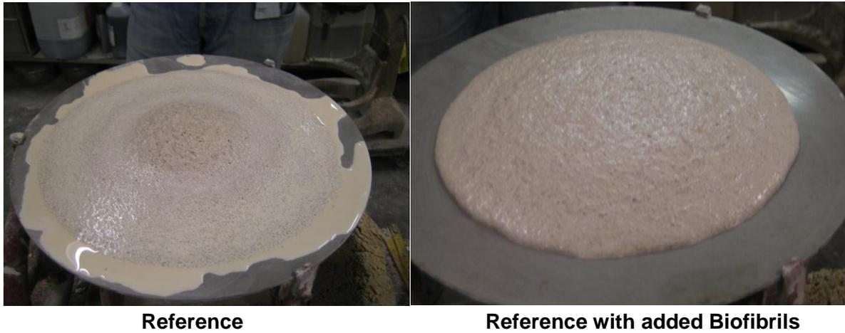
**Figure 5.** Segregation and water bleeding test with SCC using UPM Biofibrils
