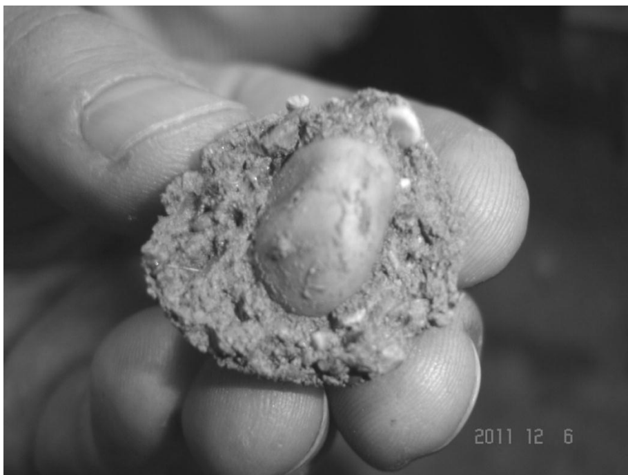
Figure 1 Typical aspect of a fresh granular material after the addition of SAP
