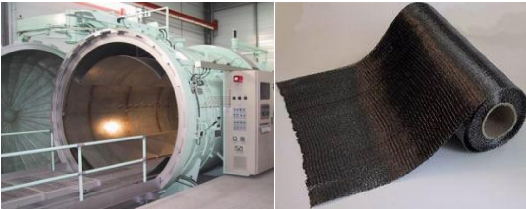
Fig. 2 - Curing oven and carbon fiber raw material
