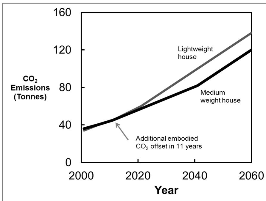
Figure 1 Cumulative CO<sub>2</sub> emissions (air-conditioned)
